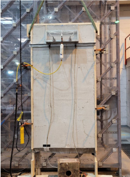
Figure 2: ASTM E2273 Test Setup at Independent, Third-Party Lab for TYPAR® BuildingWrap and TYPAR® MetroWrap
